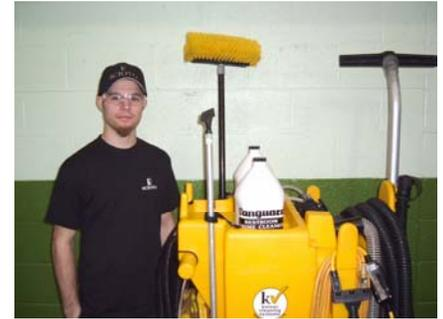
**Deep Cleaning:** Dan Napier, pictured with the Kai Vac. The Kai Vac is a "no touch" cleaning machine that can clean a restroom top to bottom. It is a combination power washer, vacuum, and blow dryer that sprays a cleaning chemical on all walls, toilets, urinals, floors and any other fixtures that need cleaned in the restroom.
